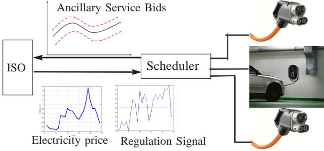
Fig. 1: Architecture of a charging station
