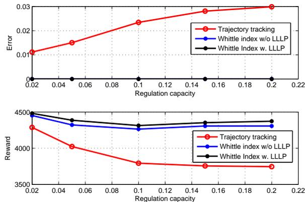
Fig. 5: Regulation signal tracking accuracy and charging reward Vs. regulation capacity.
