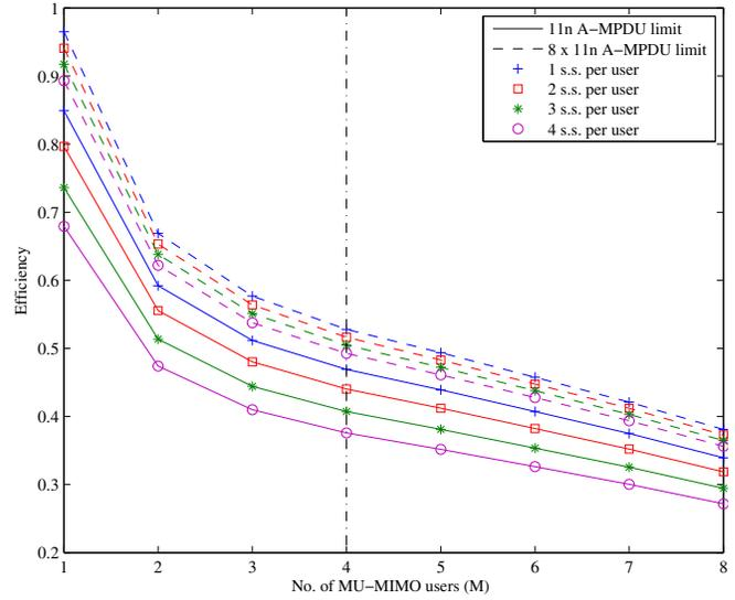
Fig. 8. Efficiency of the proposed 802.11ac WLAN in the infrastructure mode. The decrease in efficiency with  $M$  indicates the current 802.11 SU-oriented MAC cannot fully utilize the PHY layer’s MU capacity.
