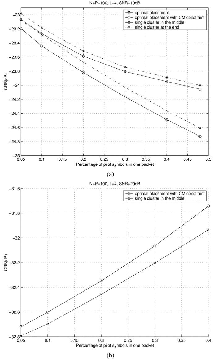
Fig. 12. (a) CRBs of different placements versus percentage of pilot symbols at  $\text{SNR} = 10$  dB. (b) CRBs versus different placements under low pilot power at  $\text{SNR} = 20$  dB.
