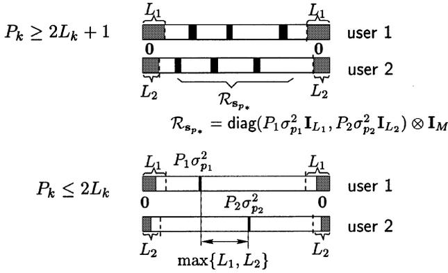
Fig. 7. Optimal placements of pilot symbols for the MIMO channel.
