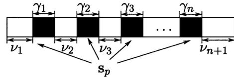
Fig. 1. Input data packet with multiple pilot clusters.
