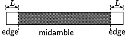
Fig. 2. Edge and midamble positions of one data packet.
