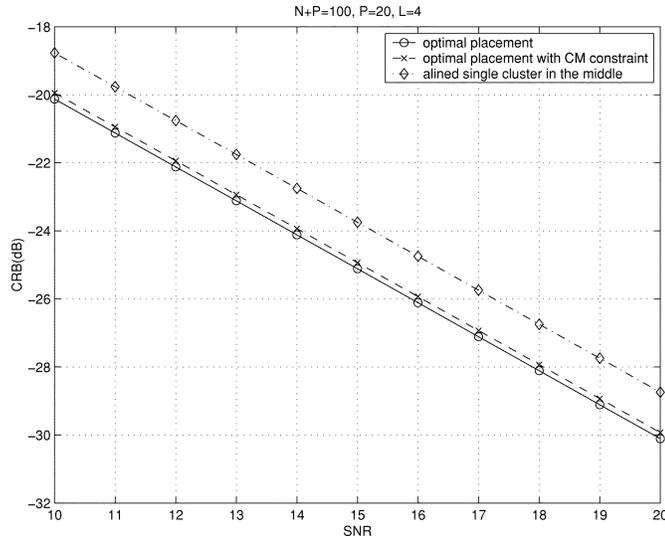
Fig. 13. CRBs of different placement schemes in a two-user case.
