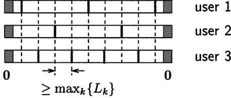
Fig. 9. Optimal placement for three-user case.
