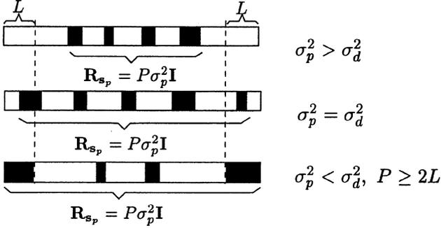
Fig. 5. Optimal placements of CM pilot symbols for SISO channels.
