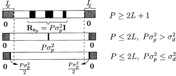
Fig. 3. Optimal pilot designs and placements for SISO channels.
