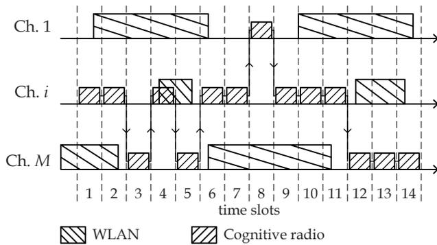
Figure 1: System setup. A frequency hopping cognitive radio coexists with a set of parallel WLAN channels.
