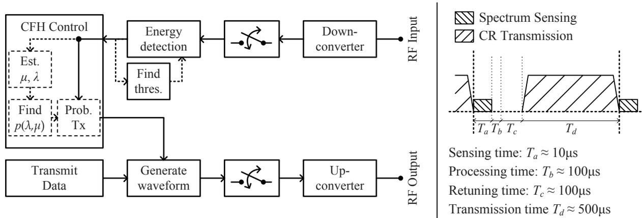
Figure 3: Block diagram of the cognitive radio (left). The slot operation and timing is shown on the right. Pictures of the cognitive radio test bed are available online at <http://acsp.ece.cornell.edu/mc2r.pdf>.
