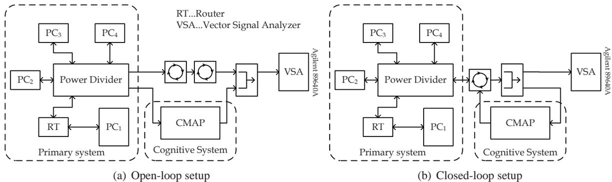
Figure 5: Measurement methodology. In the open-loop setup (left) the CR’s transmission are not fed back to the WLAN. The closed-loop setup (right) is used to quantify the impact of retransmissions.
