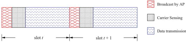
Fig. 5. Slot structure of QUIRE.
