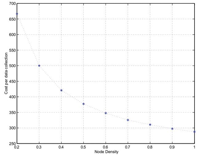
Fig. 11. Network deployment cost per IR operation ( $\omega = 1.8mJ$ ).
