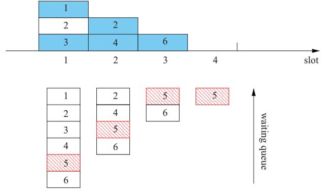
Fig. 6. Optimal cell activation of QUIRE ( $M = 6$ ,  $N = 3$ , and the 5th cell (shaded) has an empty center area). The numbered rectangles on the time axis indicate transmissions from the corresponding cells. Successful transmissions are illustrated by shaded rectangles.
