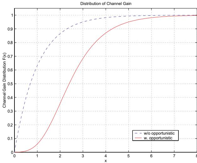
Fig. 8. Improved channel reception capability by opportunistic carrier sensing: channel gain distribution.
