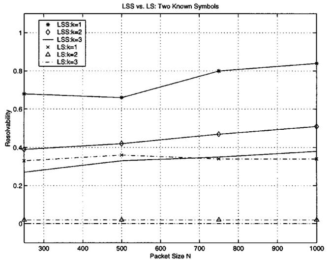
Fig. 9. Effect of packet size ( $m = 2$ ,  $q = [3, 5, 8, 10]$ , SNR = 20 dB, perfect power control).
