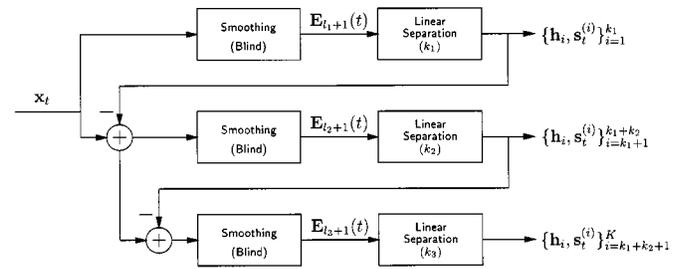
Fig. 3. Schematic diagram of the semi-blind LSS approach.
