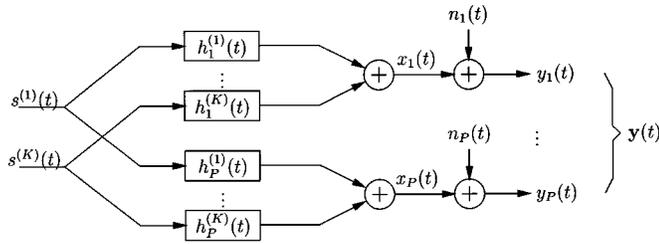
Fig. 1. Multiple-input multiple-output system.
