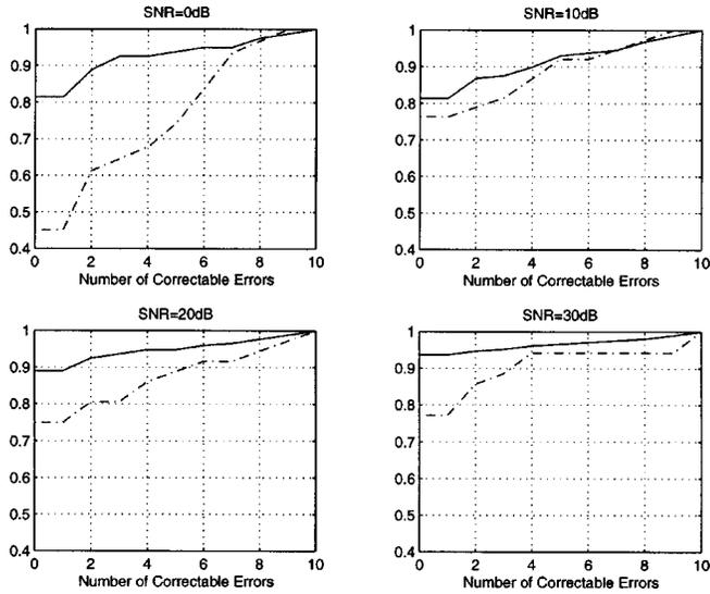
Fig. 7. Percentage of the packets detected with no more than  $q$  ( $0 \leq q \leq 10$ ) errors among the packets detected with no more than 10 errors (“-”: LSS, “—”: LS).
