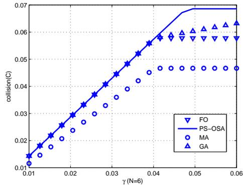
Fig. 4. The first primary user's collision probability with the secondary. The range of interference level is within the interval  $[0, 0.06]$  and  $\gamma = \gamma_i$ .
