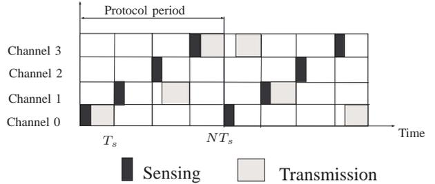
Fig. 2. Sensing and transmission structure for an  $N = 4$  channel system.
